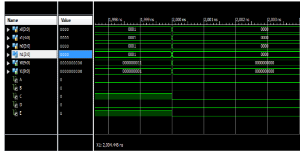
Waveform of Proposed Two- Parallel FIR Filter
